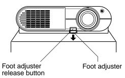
2) Turn the foot adjuster to make fine adjustment of the height.
